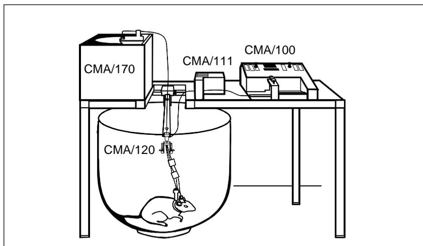
Fig. 3. The CMA/120 System for Freely-Moving Animals, CMA/100 Microinjection Pump, CMA/111 Syringe Selector and the CMA/170 Refrigerated Fraction Collector.
